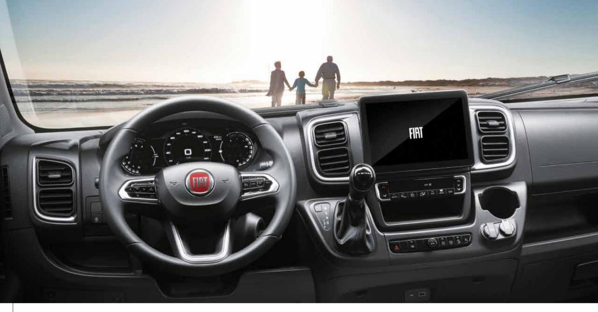
The new cluster is offered in two versions, 3,5" TFT+ analogic and 7" full digital TFT.
