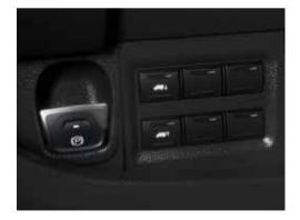
The new electric park brake provides greater comfort in everyday usage. Driver can activate holding mechanism by a dedicated switch located on dashboard; functionality can even be automatically enabled through a specific instrument cluster setting.
